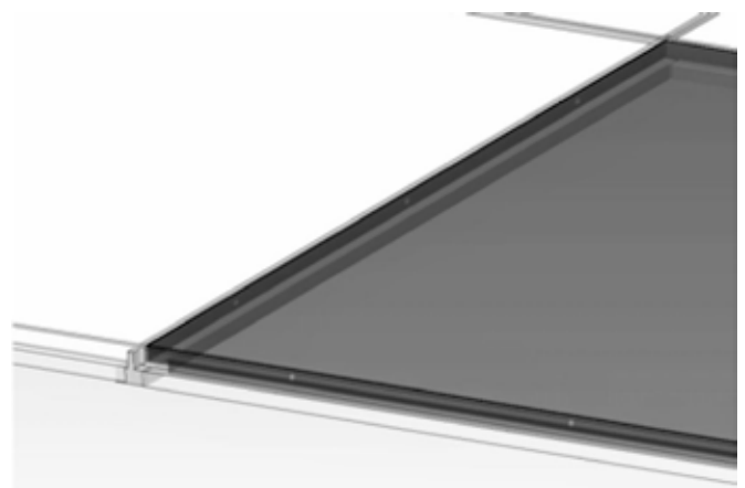
HEATING PANEL INSTALLED ON THE METALIC FRAME OF THE CEILING
