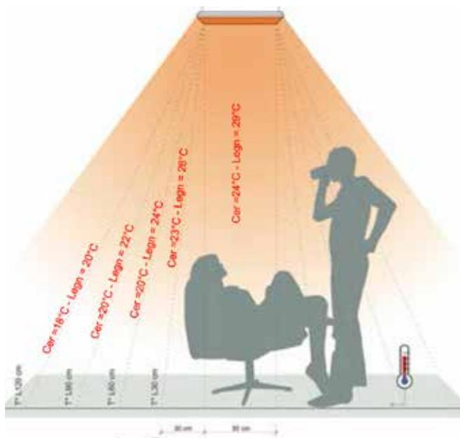
INSTALLED RADIANT PANEL H. 2,70 m - 106.29 in
