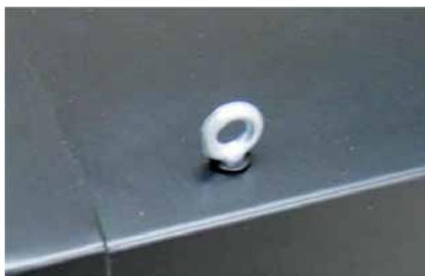
ONE OF FOUR FIXING RINGS LOCATED ON THE PANEL'S CORNERS
