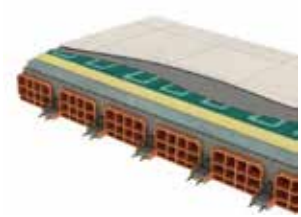
MESH BETWEEN INSULATION PANEL AND FLOORING
