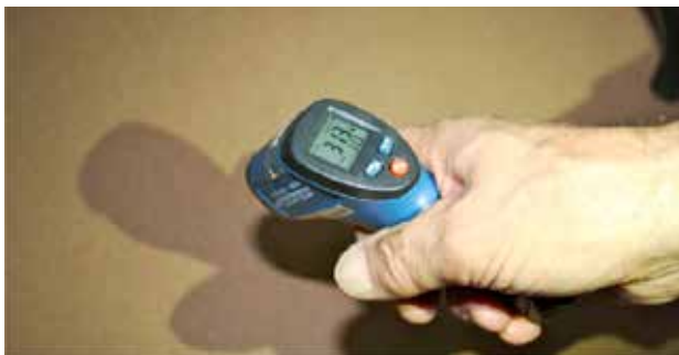
SURFACE TEMPERATURE CHECKING
