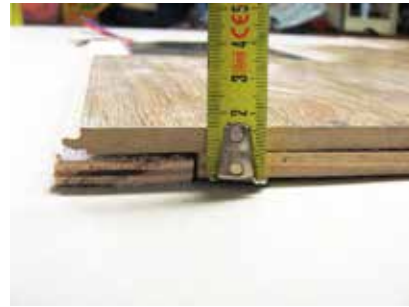
ENTIRE THICKNESS INCLUDING LAMINATE (1,80 mm/0.63 in)
