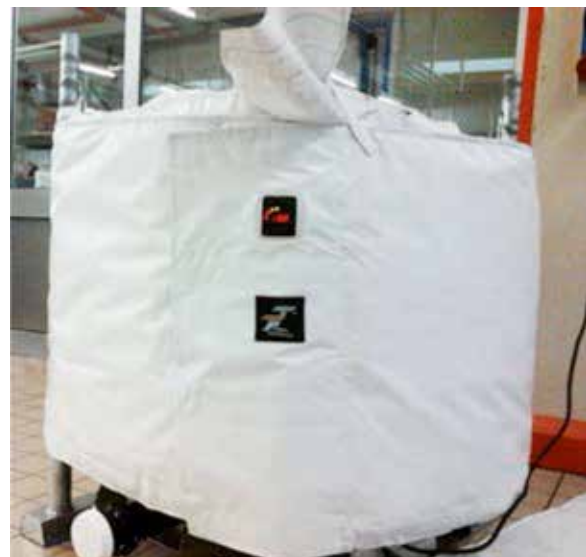
HEATING BLANKET MOUNTED ON THE "FLUID-BAG" CONTAINER
