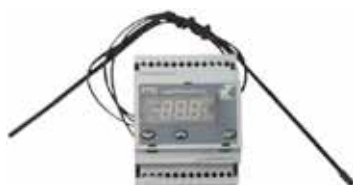
T751 TEMPERATURE CONTROLLER
