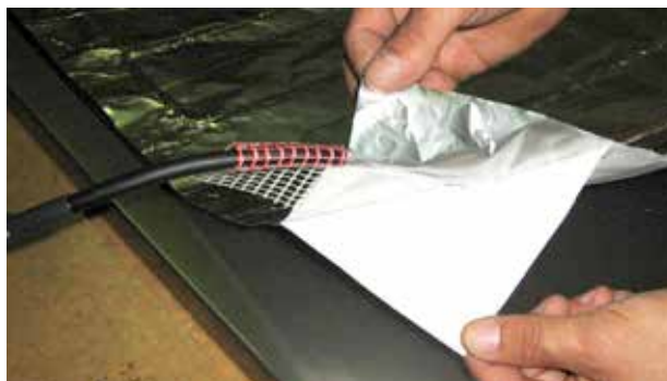
REMOVAL OF THE PROTECTION FILM FROM ADHESIVE ALUMINIUM
