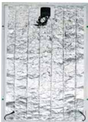
HEATING SHEET APPLIED ON THE REAR SIDE OF A PHOTOVOLTAIC PANEL
