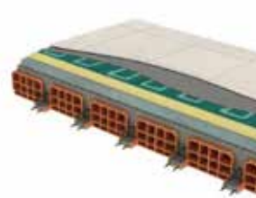
MESH BETWEEN INSULATION PANEL AND FLOORING
