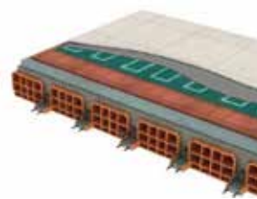
MESH BETWEEN OLD AND NEW FLOORING
